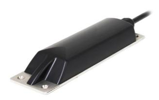
The BELUGA<sup>TM</sup> is the newest ultrasonic Doppler area/velocity flow meter sensor for open channel flow measurements from Flow-Tronic. The new sensor combines advanced digital Doppler ultrasonic velocity sensing technology with most modern and powerful DSP processor technology allowing real-time spectral analysis of the velocity distribution through the cross-sectional area.
