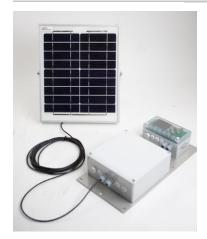
Metron4/S/SOL SYS runs from a 10 Watt solar power and lead acid battery via an intelligent charge regulator.
