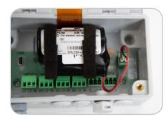
Ensure the SIM card is installed. Plug in the power source.
