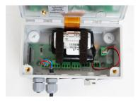
Plug the connector into the correct input channel and tighten the gland. Ensure cable is through the gland.
