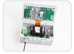
Insert connector into plug in terminal connector
