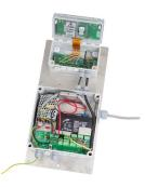
UPS 12 V Uninterruptable power supply is a separate box (262 × 188 mm). Mains 110 / 230 Vac in 12 Vdc maintained output via battery backup. Battery can typically support 50 transmissions. IP54 protection rating. Run cable from UPS 12 V to Metron4.
