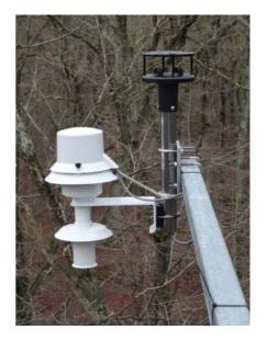
Data collected from the WindSonic anemometers are used to estimate the wind velocity gradient and wind direction shear in the forest vertical profile and to determine the air turbulences in the plant cover. Furthermore the data associated to air humidity measurements is also used to calculate the real evapotranspiration of the forest ecosystem.
